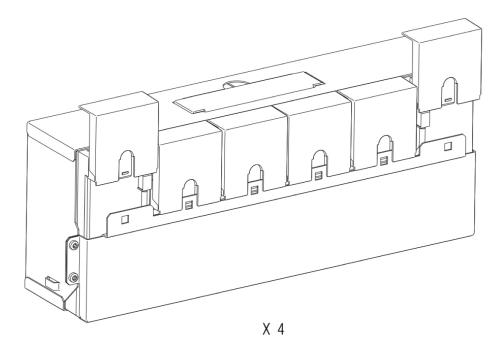
Add two battery blocks on a drawer and connect in series the two blocks using the cable provided and respecting the polarity (connect a positive terminal to a negative terminal).
