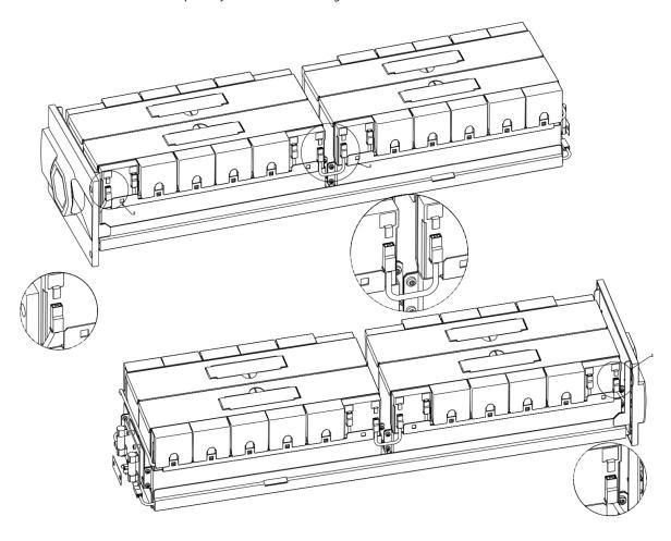
Insert the remaining terminal covers on the batteries.
