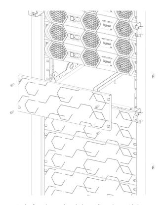
Insert the empty battery drawers in the free slots and push them till you hear a 'click'. The battery blocks must be added to the drawers only when these are inserted in the cabinet.
