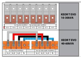
Connect the phase cables to X1 MAINS SUPPLY: X1/L1 - X1/L2 - X1/L3 terminals, the neutral to X1 MAINS SUPPLY: X1/N terminal.
