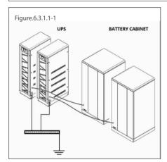
Input Mains Supply's Protective Earth terminal **PE** of the UPS shall be connected to the ground with a low impedance connection.
