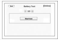
With this command, UPS battery test feature can be started. When you touch the **Start test** key, a confirmation pop-up bar will appear.
