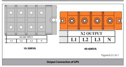
Connect the phase cable to X2 OUTPUT: X2/L1 – X2/L2 – X2/L3 terminal and the neutral cable to X2 OUTPUT: X2/N terminal.
