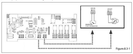
UPS output can be switched off immediately by Remote Emergency Switching Device interface (ESD) connection if desired. A remote latched switch can be used as described in above figure.
