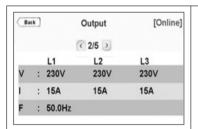
Output voltage (Ph-N), current, frequency information of each phase is displayed.
