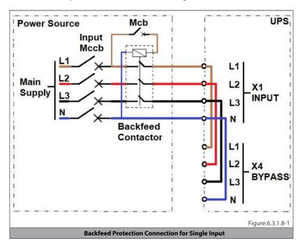
The external device (contactor) is not part of the UPS, is provided and installed at customer care.
