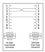
If Serial Communication cable is needed, it can be produced according to the pin configuration described at side.
