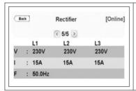
Rectifier voltage (Ph-N), current and frequency information of each phase are displayed. If the MAINS and AUX Supply are connected in COMMON, Rectifier and Bypass values will be the same.
