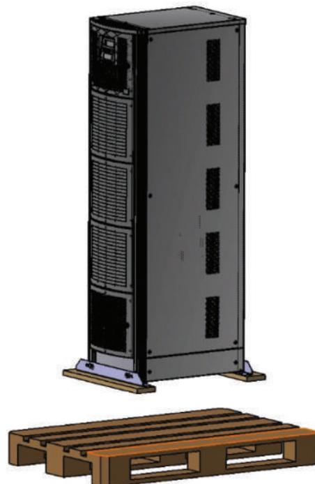
5. Remove the front and rear brackets from the UPS by unscrewing the retaining screws
