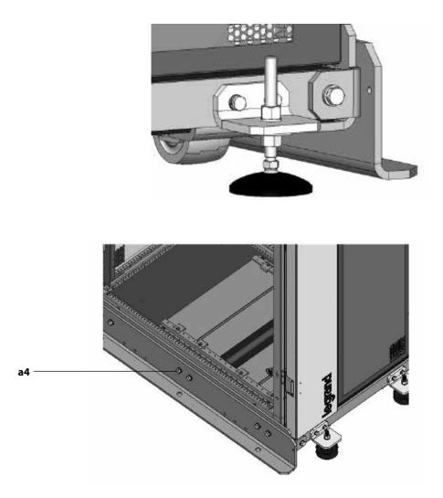
Only for the 3 111 19 (Keor MOD 125 kVA), in addition to the seismic basement, there are also ten metal bars and twenty M4x8 screws to keep stable the battery packs in the drawers. For each battery drawer, after having followed the instructions in the Keor MOD installation manual to install the battery packs, mount a metal bar with two relative screws as shown in the picture:
