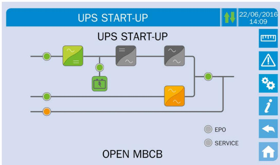
Picture 21 – Opening the manual bypass switch
