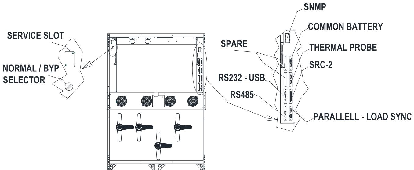
*Picture 8 – Position of the serial interfaces of KEOR HPE 400-500 kVA*
