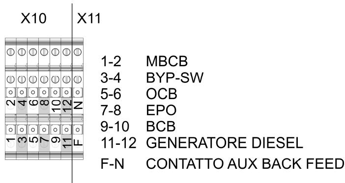
Figura 7 – Morsetti ausiliari KEOR HPE 400-500 kVA
