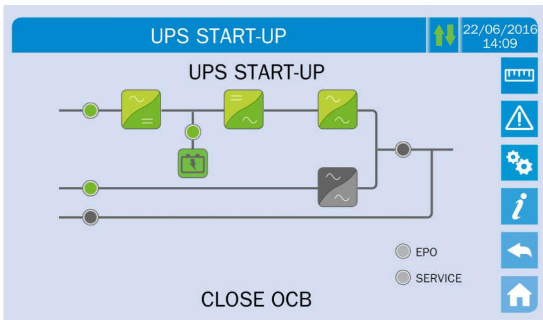
Picture 15 – Connecting the UPS to the load
