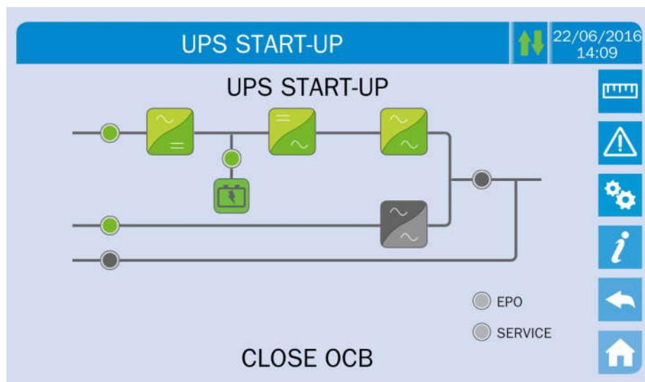
Illustration 15 – Connecting the UPS to the load
