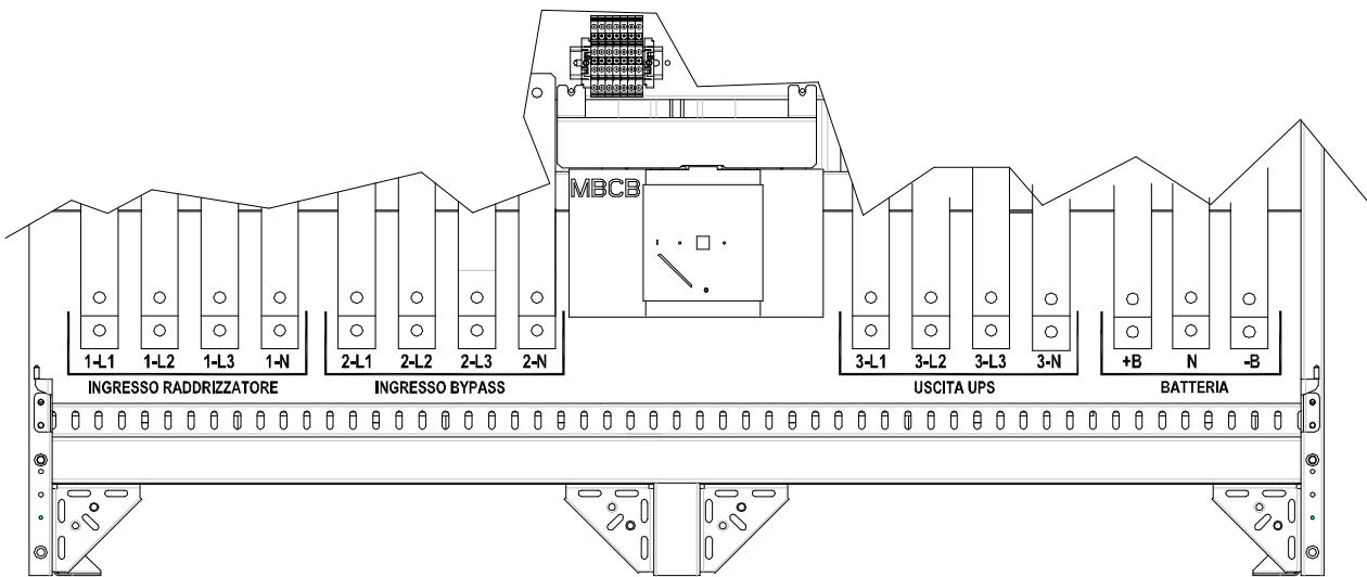
Figura 6 – Morsettiera KEOR HPE 400-500 kVA
