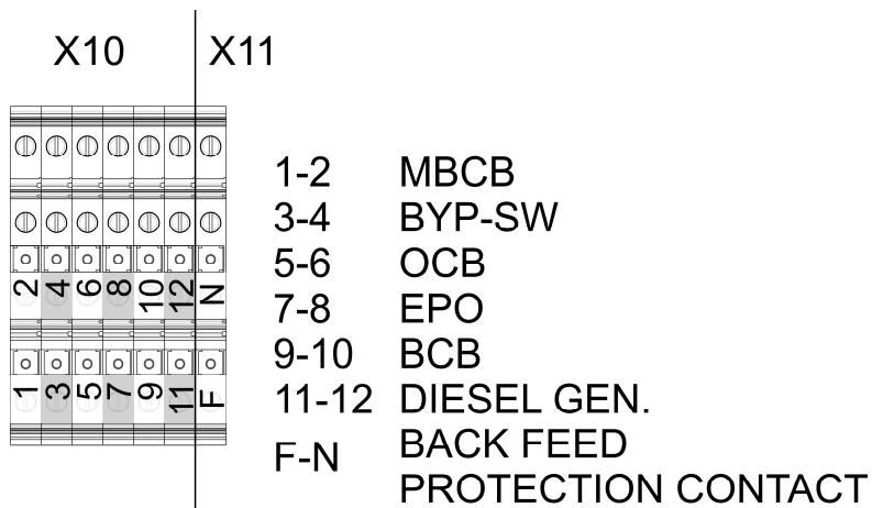
Picture 7 – Auxiliary terminals of KEOR HPE 400-500 kVA
