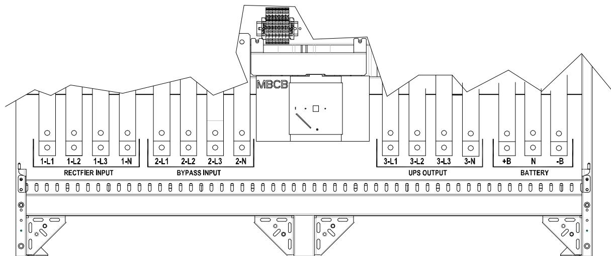
Picture 6 – Terminal board KEOR HPE 400-500 kVA
