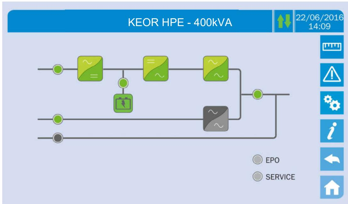
Picture 24 – Re-start from manual bypass completed
