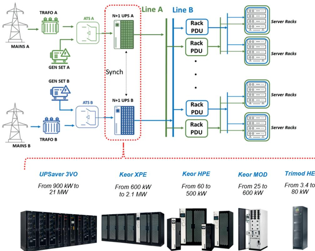
Datacenter with line A and B (level of redundancy 1) and N+1 (level of redundancy 2) both with modular and conventional UPS
