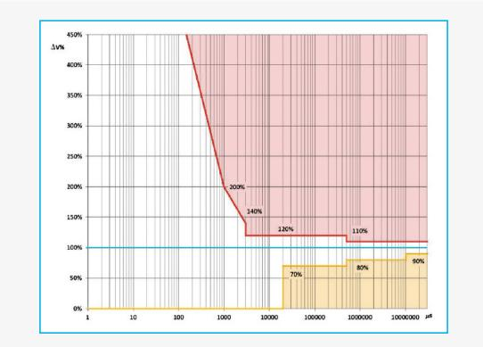
ITIC curve: the area in WHITE represents all of the combinations of variations in supply voltage and duration, in which the electronic device does not experience any changes in operation.
