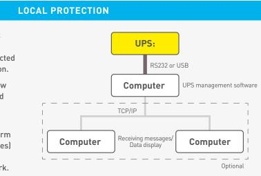
You can simply use an RS232 or a USB connection and install management software on the computer being protected to provide one single layer of protection.
