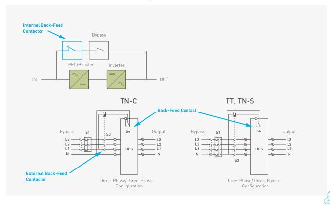
The two cases of internal and external back feed protection are illustrated below:
