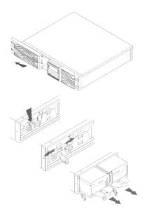
Internal batteries UPS Daker DK Plus 1-2-3 kVA Online Double
